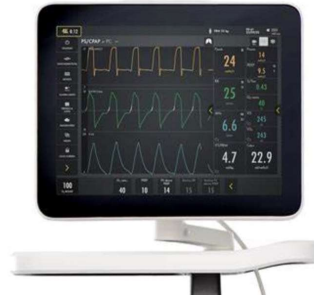
PICU Servo U Dual limb circuit. Can be used for HF/ BiPAP/invasive ventilation
